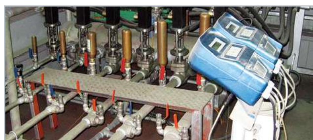
[Figure 4] Equipment for testing impact absorbing capability
